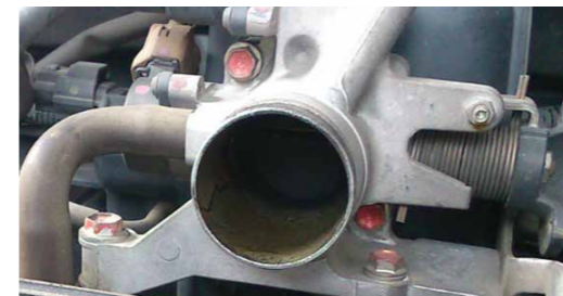
BEFORE (Throttle body condition after 60,000 km)
